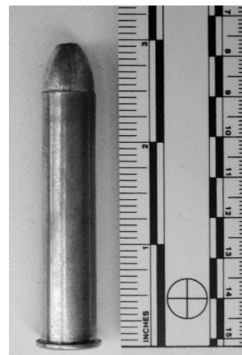
The .50-90 Sharps rifle is referred to as a Big Fifty. The cartridge is a .50 caliber bullet loaded in a 2.5-inch length cartridge case and loaded with 90 grains of black powder. (Photograph by authors)
