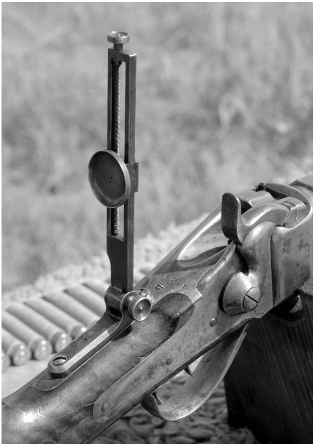
Tangent peep sight with vernier adjustments for elevation and windage. (Photograph by authors)
