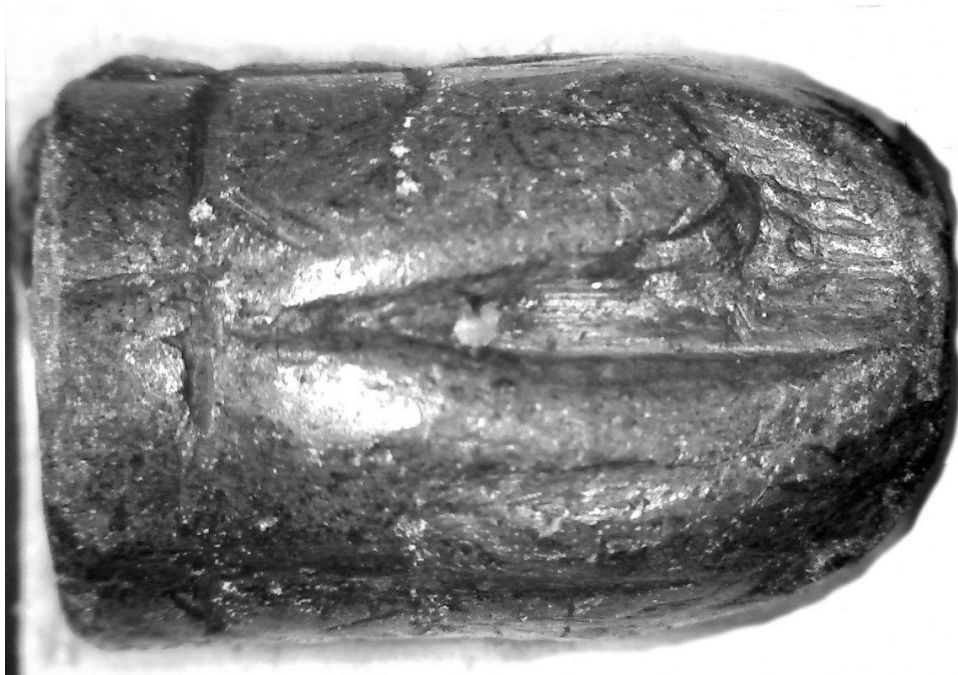
Nose Deformation on Acme Saloon Bullet. (Authors' Collection)
