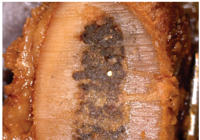
Figure 14: Sample after 6 months in 5% iodine solution
