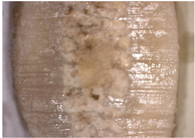
Figure 18: Sample after 6 months in 6% sodium hypochlorite
