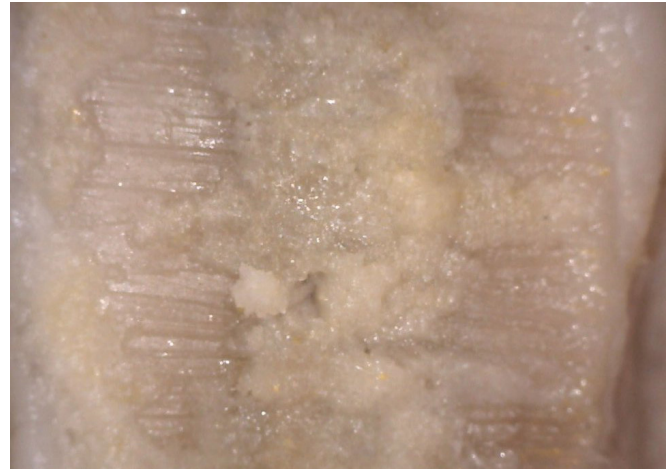
Figure 4: Sample after 6 months in buffered 10% formalin
