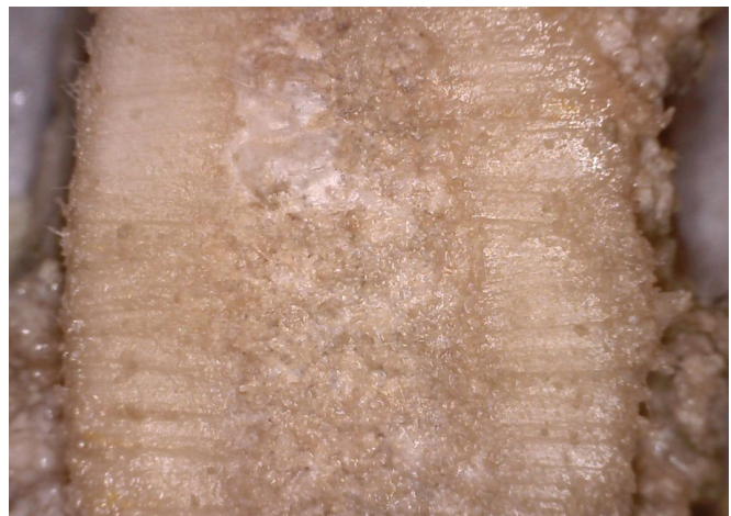
Figure 20: Sample after 6 months in 10% NaCl with iodide
