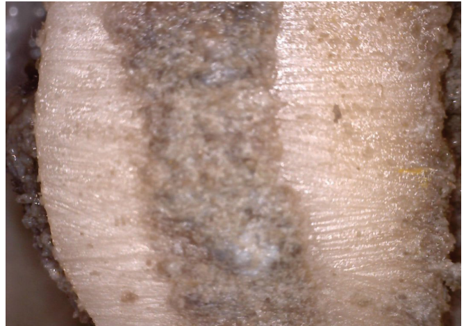
Figure 22: Sample after 6 months in 10% NaCl, no iodide
