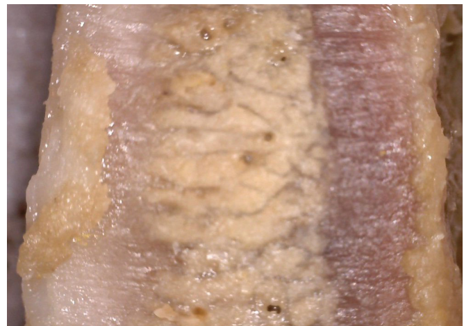
Figure 8: Sample after 6 months in 70% isopropyl alcohol
