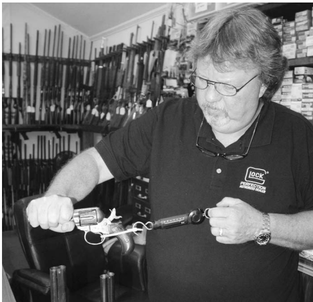
Alan Tiller conducts trigger pull test on Colt Thunderer to determine the number of pounds needed to fire the double action revolver. (Photo by authors)
